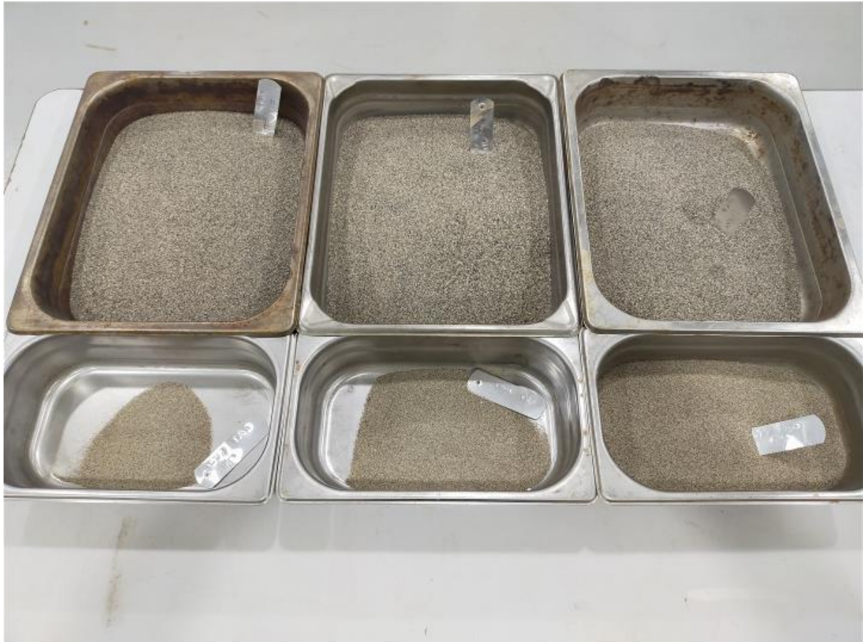
Plate 4 - Construction sand samples from large scale pilot plant program used in concrete mix testing.
