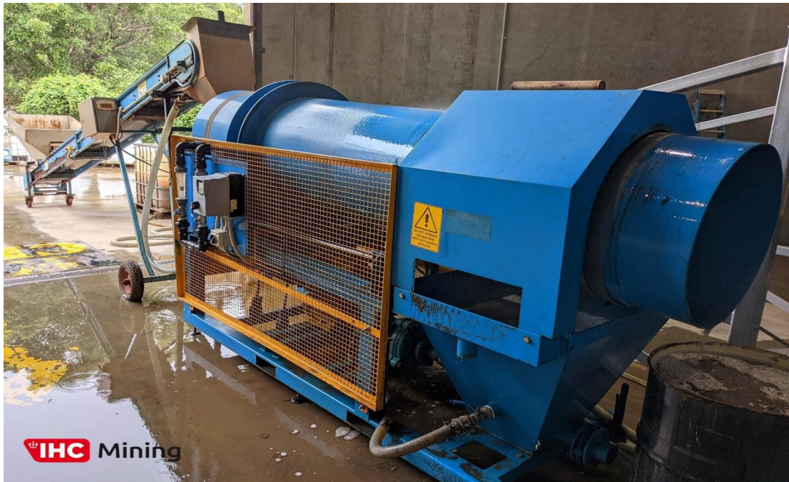
Plate 2 – Trommel used for oversize and trash removal (>2mm)
