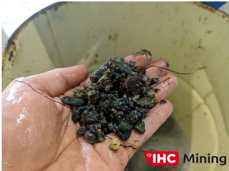
Plate 3 – Pebbles and organic matter from Trommel
