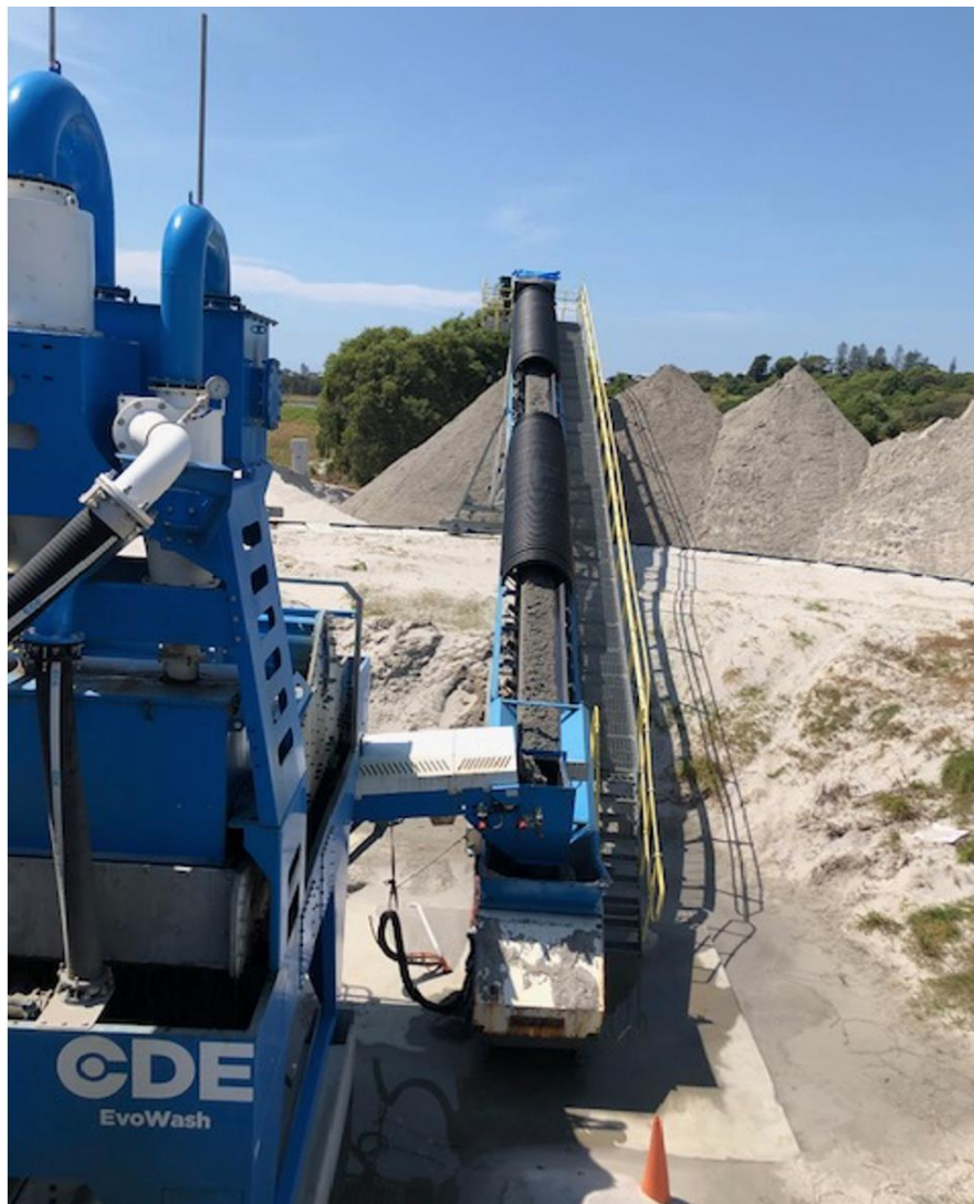
Plate 9 - Dewatered sand and movable stacker
