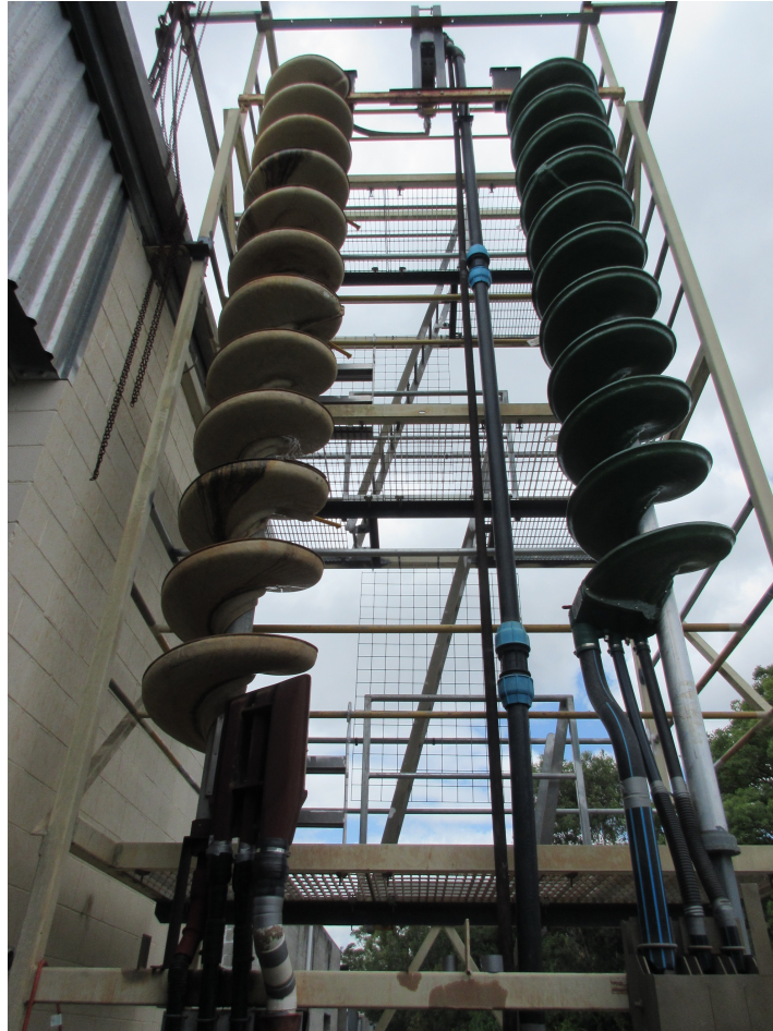
Plate 1 – Spiral bank used to separate heavy minerals from lighter sand during pilot plant tests at IHC Robbins metallurgical facility.
