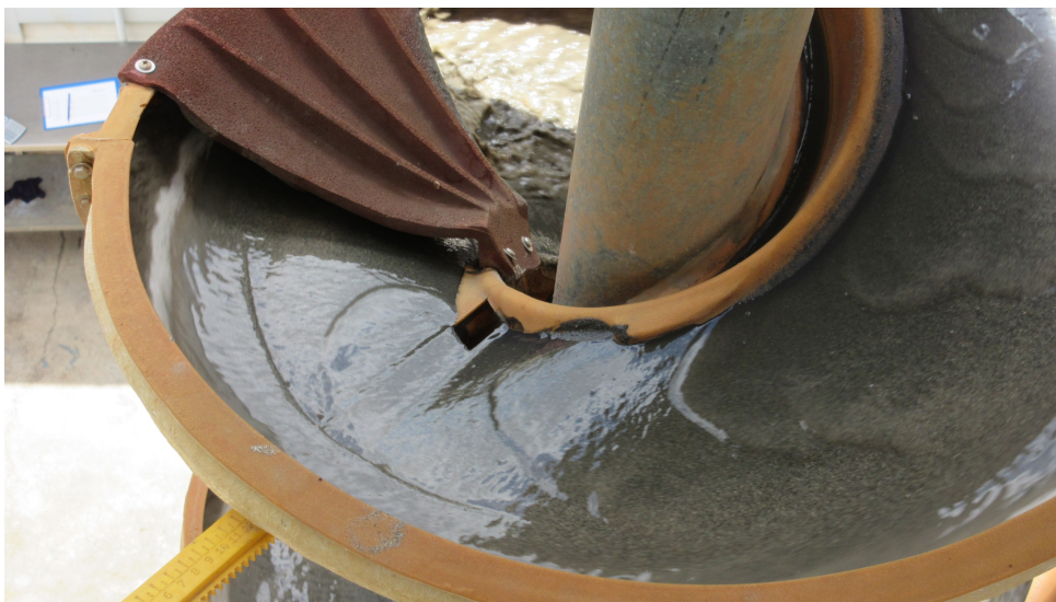
Plate 2 – Darker heavy minerals (including magnetite) concentrate toward the spiral centre where they are selected for recovery
