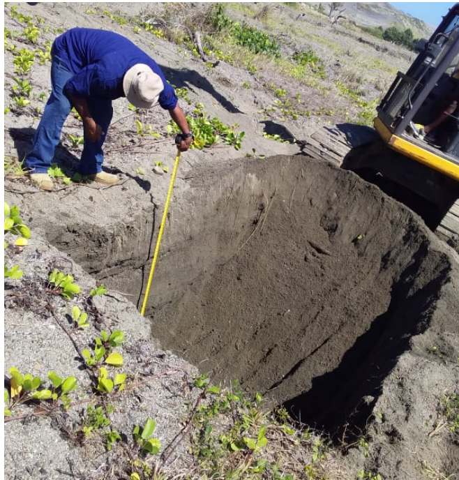
Plate 2 – Depth measurement prior to sample collection
