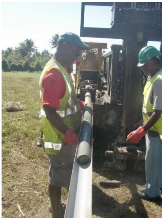
Figure 1: Sonic Drill Rig and the high quality soft ‘core’ it generates.
