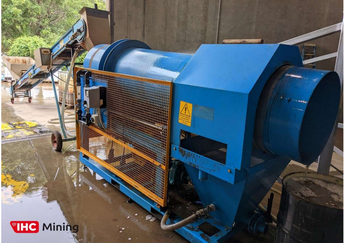
Plate 2 – Trommel used for oversize and trash removal (>2mm)
