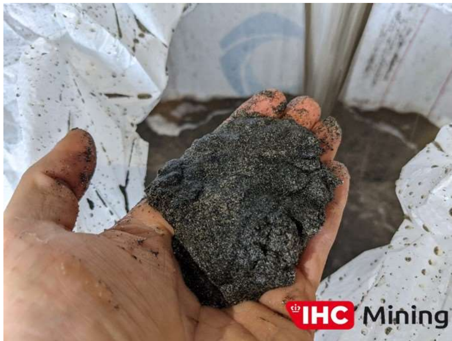
Plate 5 – Washed sand ready for industrial sand and magnetite-heavy mineral recovery (+2mm -45 \mu\text{m} )
