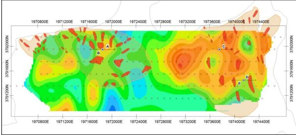
**Figures 6 & 7 –** Plots of the chargeability (top) and resistivity responses at an apparent depth of 250m with the outline of the argillic (hatch) and silicification (red) superimposed as well as locations recommended for exploration drilling.
