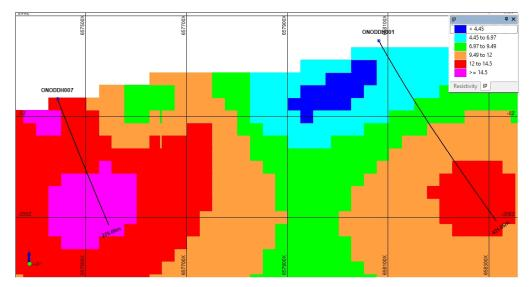
**Figure 8 –** IP chargeability cross-section, section showing the trace of drill holes ONODDH001 and 7. These holes tested the high chargeability anomalies (red/purple zones) in the lower part of the hole.
