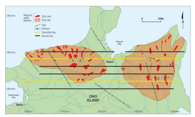
**Figure 5 –** Naqara East and West Prospects on Ono Island showing the extent of hydrothermal alteration and the IP survey lines. Proposed drill hole locations (A to E) are based on the IP results and surface geology
